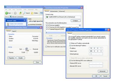
The network connection configuration screen in Windows XP being configured to communicate with an IOtech Ethernet-based data acquisition system.
